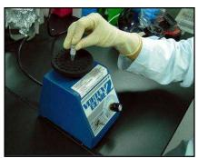
Gently tap the tubes several times (hereinafter referred to as "tapping"), or vibrate the tubes 3 times for approximately 1 second on a vortex mixer. After the mixture becomes homogenous, centrifuge the tubes to collect the solution in the bottom of the tubes (hereinafter referred to as "spin down"), and then put the reagents on ice.
