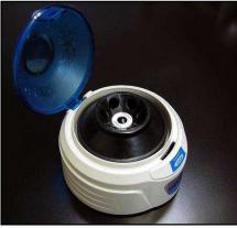
• Centrifuge for test tube
