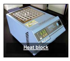
Close Test Tube and mix the reagents by tapping or vibrating on a vortex mixer for about 1 second x 3 times, and spin down the tube. Incubate Test Tube at  $63^{\circ}$ C for 60 minutes in the incubator (Air incubator, heating block, or water bath).
