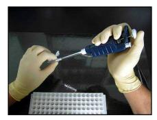
To make <u>Test Solution</u>, add TYLCV Detection Solution, Fluorescent Detection Solution, and TYLCV Enzyme Solution to a sterilized microtube (1.5 ml or 2.0 ml). Mix the reagents by tapping or vibrating 3 times for approximately 1 second on a vortex mixer, and spin down the tube. Place the tube on ice. Refer also to the following table.
