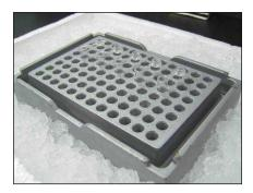
Pick a Test Tube out from the bag with a clean tweezer. Dispense 23.0  $\mu$ l of <u>Test Solution</u> into each Test Tube.
